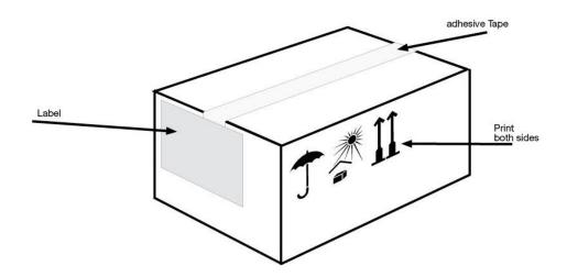
If not despatched as individual cartons final pallet preparation ensures that there is no mixed content unless agreed and the *EURO* pallet dimensions are 800mm (W) x 1200mm (L) x 2000mm (max. height) with a max. weight of 500 Kgs.
