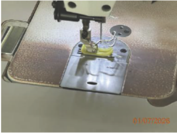
corrective action taken photo - needle guard was installed in the sewing machine.JPG
