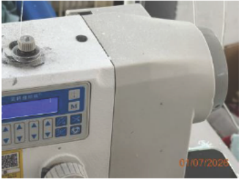
corrective action taken photo - pulley guard was installed in the sewing machine.JPG
