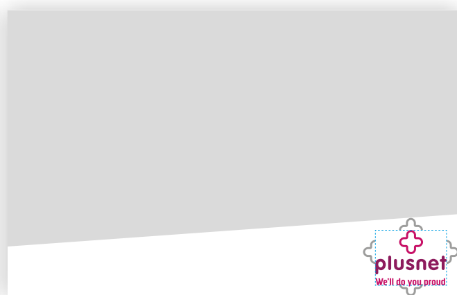
Step 4: The logo Dividing the diagonal measurement by 10 provides you with the height of the logo. Multiplying the border width by 1.5 provides the positioning of the logo from the right. Using the logo's exclusion zone provides the height of the bottom panel.
